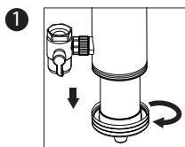
Twist off the filter base and remove the expired filter.
