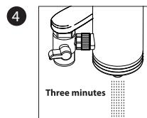
Switch the lever to the level position and flush for 3 minutes.
