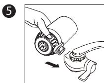
Align the slot of filter base with the slot of mounting base.
