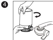
Twist the filter top cover on.
