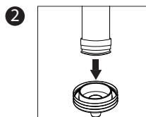
Take out the new filter and press it into the filter base . Ensure the sealing ring is in place.
