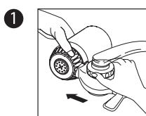
Twist the Filter Base from the Mounting Base.
