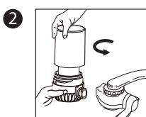
Twist the filter top cover off and take out the old filter.
