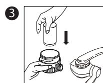
Insert new filter into the filter base.
