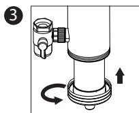
Twist the filter base with the filter top cover .
