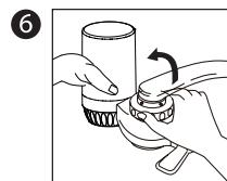
Insert filter base into mounting base and rotate 90° upward.
